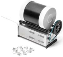
The **barreling machine** or barrel polisher consists of a barrel shaped container which sits on top of a motor and is rotated. The jewellery pieces are placed inside the barrel, with steel shot, water, and barreling solution. The barrel rotation will polish the jewels.
