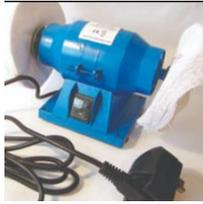
A second technique is to use **polishing compounds** which have minuscule abrasive particles held together in a binder. There are many kinds of these compounds which can be applied with a brush.
